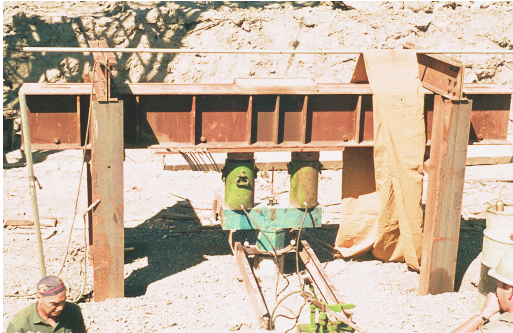
Figure 4. Photo of test arrangement for the precast pile (photo by B.H. Fellenius)
